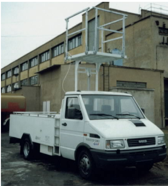
Picture showing, portable water truck with a forward mounted lift on a IVECO Turbo Daily chassis
